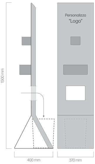
Material: Inox AISI 304 thickness 1,5 mm Total size: 370 x 400 h 1500 mm Gel dispencer dimensions: 100 x 100 h 85 mm Gloves holder dimensions: 250 x 125 h 100 mm Net weight: 12 Kg (no basket) Packaging: carton box
